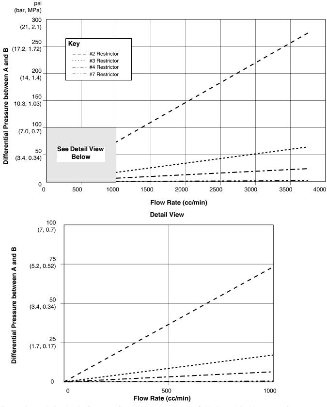
FIG. 22. Dynamic Dosing Performance (20:1 Ratio, 90 centipoise fluid, 100 psi A side pressure)
